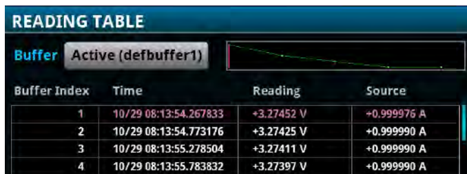
FIGURE 9. The results of five repeated forward voltage tests on a high brightness LED.
