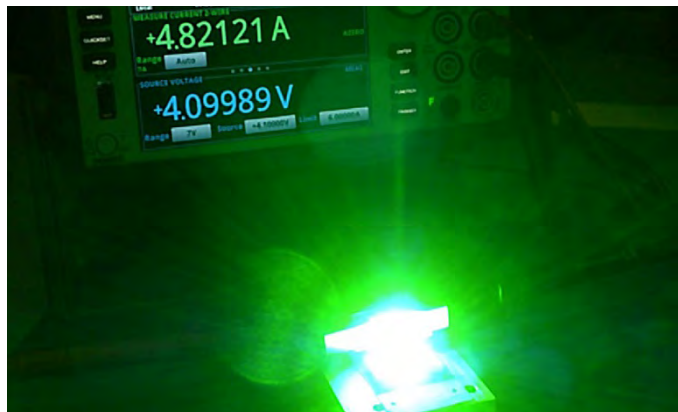
FIGURE 13: HBLED illuminated at 4.1 volts and 4.8 amps.
